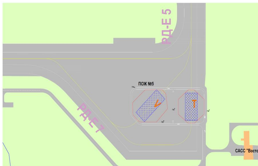
Figure J.5. Layout scheme of the AIF "W" (PL Nos. 7A, 9A); AIF on TW S1, TW S2, TW S8 pads for de-icing of the aircraft with the engines running in the western part of the STC ramp
